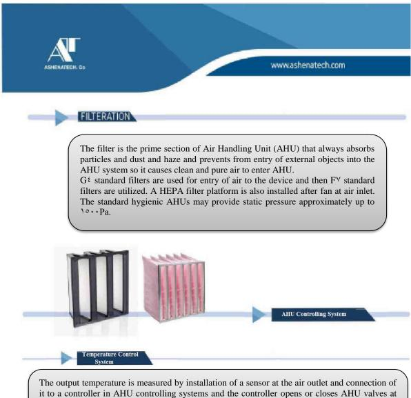
it to a controller in AHU controlling systems and the controller opens or closes AHU valves at certain levels with respect to the determined air temperature. Likewise, the feedback of changes in input temperature to the air of room is visible by connecting room thermometer to the controller.
